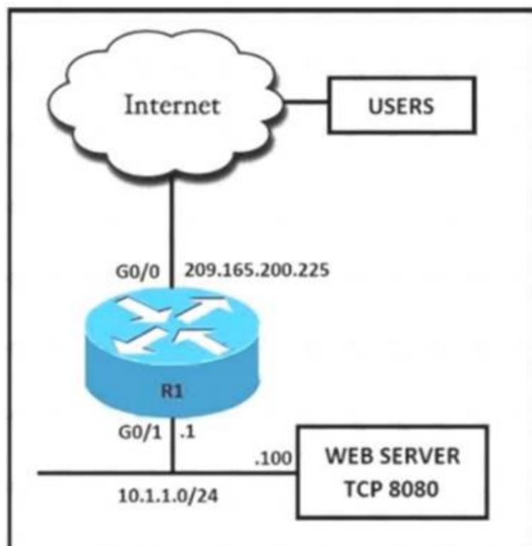
External users require HTTP connectivity to an internal company web server that is listening on TCP port 8080. Which command set accomplishes this requirement?
