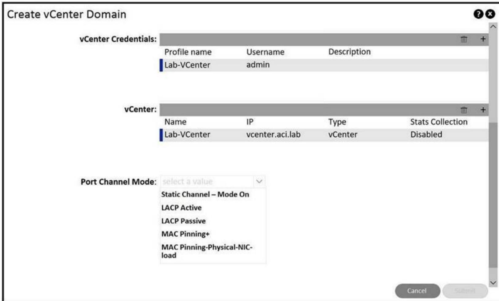
An engineer is implementing Cisco ACI – VMware vCenter integration for a blade server that lacks support of bonding. Which port channel mode results in “route based on originating virtual port” on the VMware VDS?
