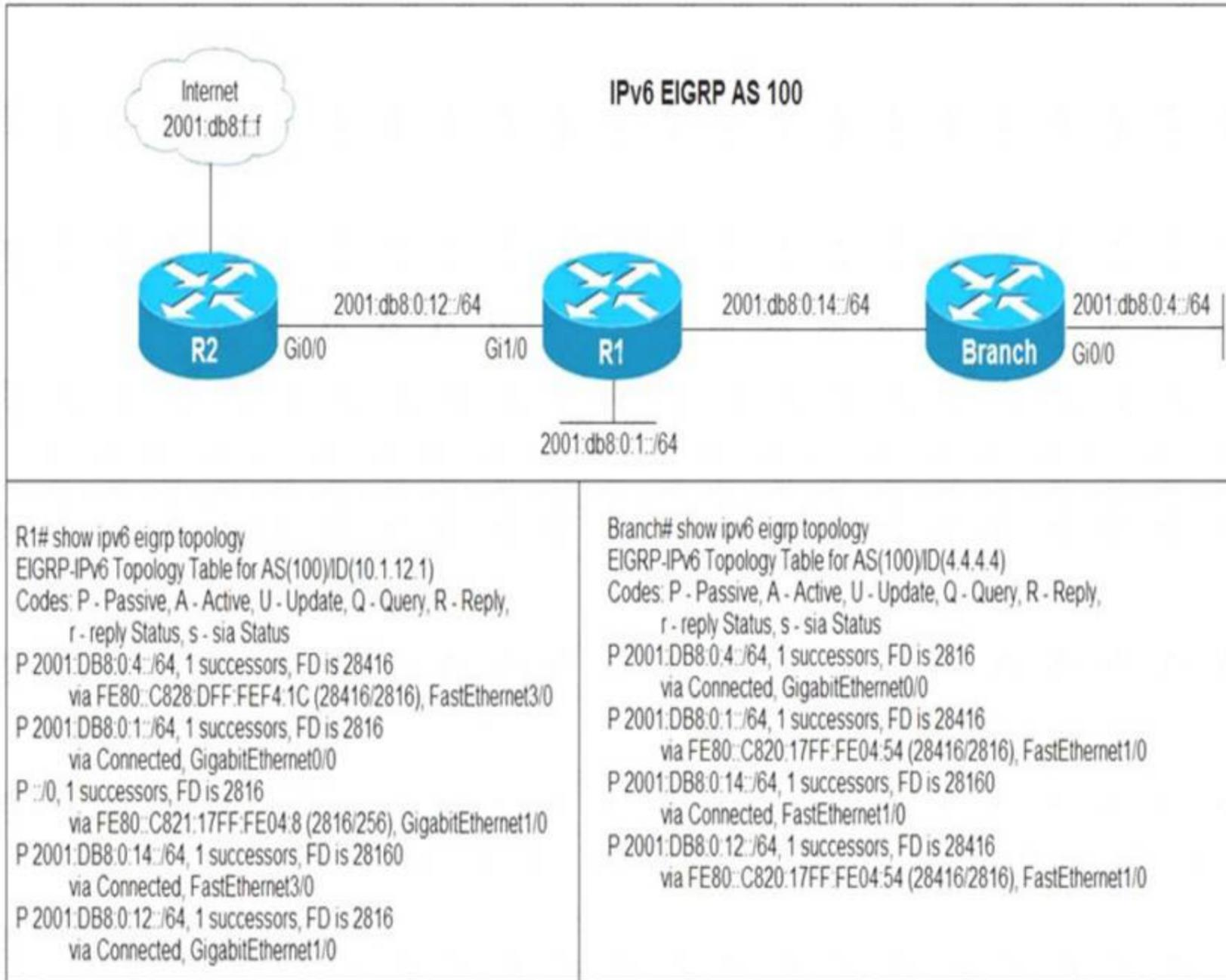
Users in the branch network of 2001:db8:0:4::/64 report that they cannot access the Internet. Which command is issued in IPv6 router EIGRP 100 configuration mode to solve this issue?
