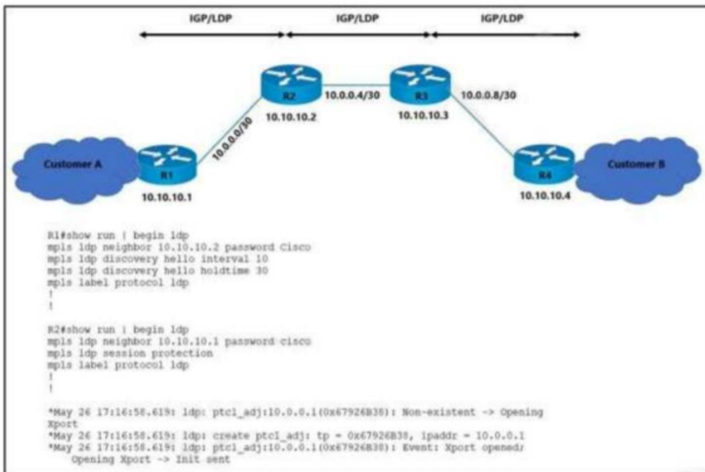
The operations team is implementing an LDP-based configuration in the service provider core network with these requirements: R1 must establish LDP peering with the loopback IP address as its Router-ID. Session protection must be enabled on R2. How must the team update the network configuration to successfully enable LDP peering between R1 and R2?
