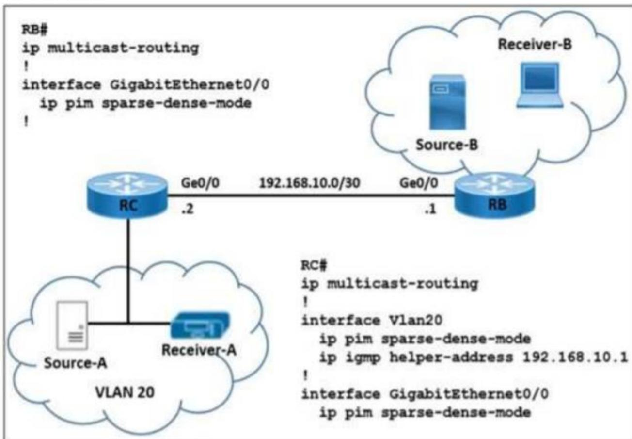
A network engineer is implementing multicast Source-A to send a multicast stream for Receiver-A, and multicast Source-B to send a multicast stream for Receiver-
