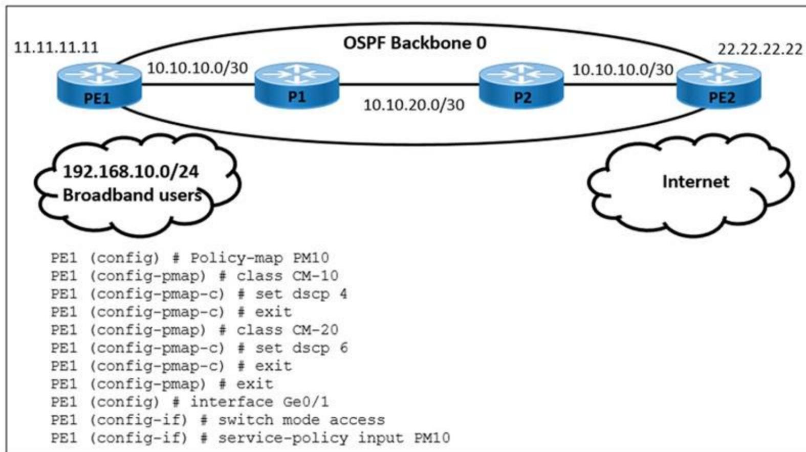
A user is performing QoS marking on internet traffic and sending it with IPv4 and IPv6 headers on the provider edge device PE1. IPv4 traffic is classified with DSCP 4 and IPv6 traffic is classified with DSCP 6. Which action must the engineer take to begin implementing a QoS configuration on PE1 for the IPv6 traffic?
