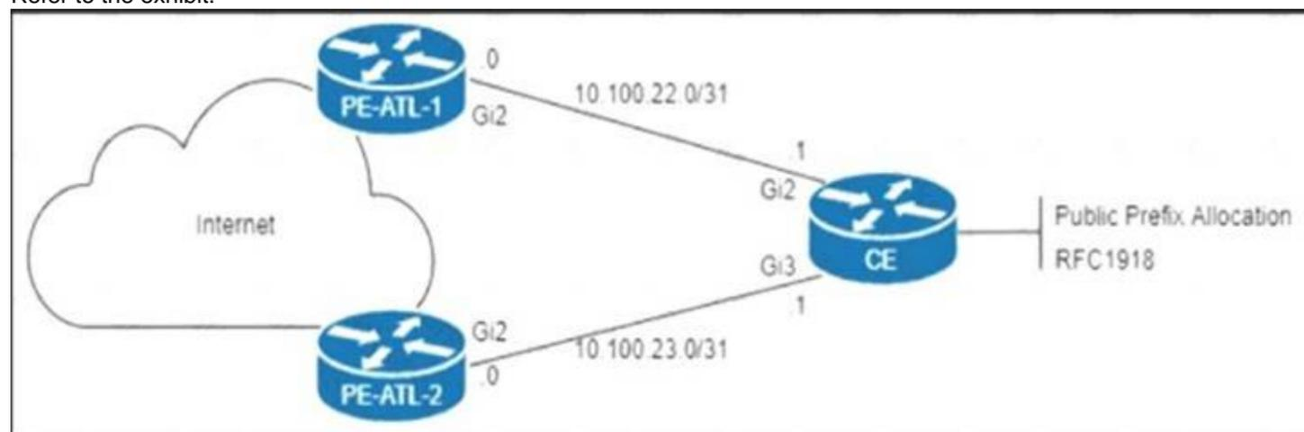
The CE router is peering with both PE routers and advertising a public prefix to the internet. Routing to and from this prefix will be asymmetric under certain network conditions, but packets must not be discarded. Which configuration must an engineer apply to the two PE routers so that they validate reverse packet forwarding for packets entering their Gi2 interfaces and drop traffic from the RFC1918 space?
