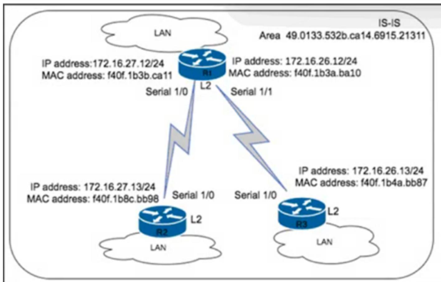
An engineer with an employee 10:4350:47:853 is implementing IS-IS as the new routing protocol in the network. All routers in the network operate as Level 2 routers in the same private autonomous system, and the three branches are connected via dark fibre. The engineer has already implemented IS-IS on router R1 with NET address 49.0133.532b.ca14.6915.21311.F40F.1B3a.ba10.00. Which IS-IS NET address configuration must be implemented on R3 to establish IS-IS connectivity?
