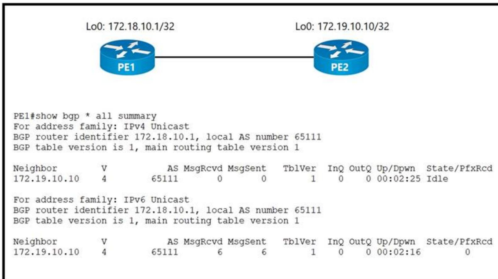
An administrator working for large ISP must connect its two POP sites to provide internet connectivity to its customers. Which configuration must the administrator perform to establish an iBGP session between routers PE1 on POP site 1 and PE2 on POP site 2?
