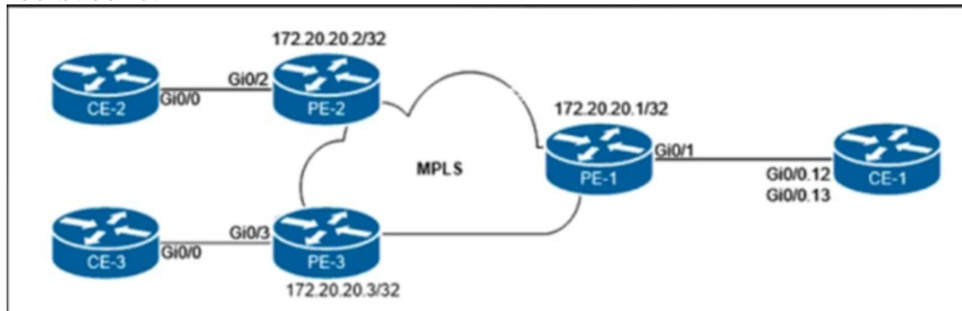
The customer that owns the CE-1, CE-2, and CE-3 routers purchased point-to-point E-Line services from the Carrier Ethernet provider. The service provider is delivering multiplexed UNI at the customer HQ location on PE-1 and untagged UNIs at the PE-2 and PE-3 locations. Additionally, the customer provided these VLAN to EVC mapping requirements:
