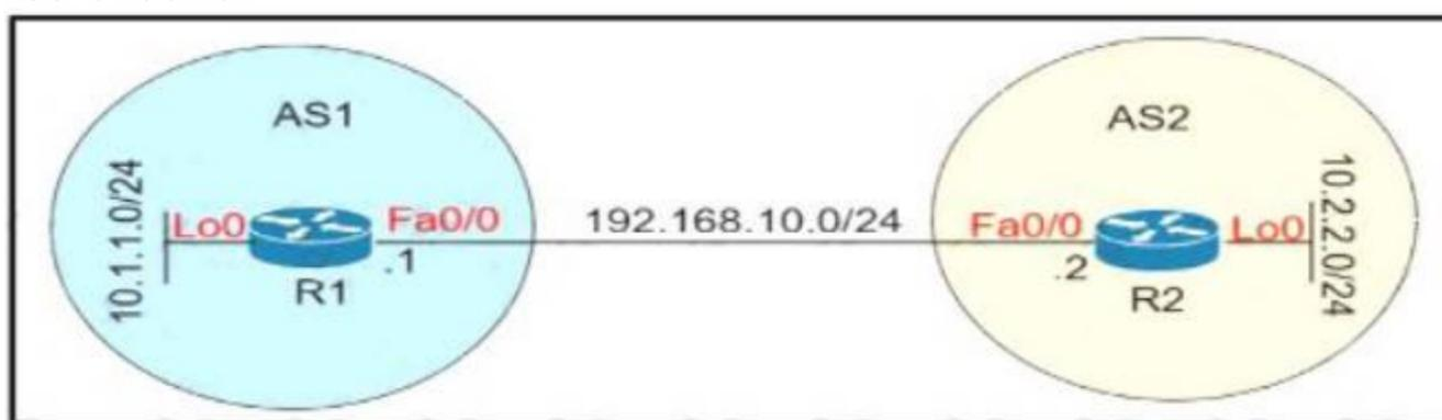
Which configuration establishes EBGP neighborship between these two directly connected neighbors and exchanges the loopback network of the two routers through BGP?
